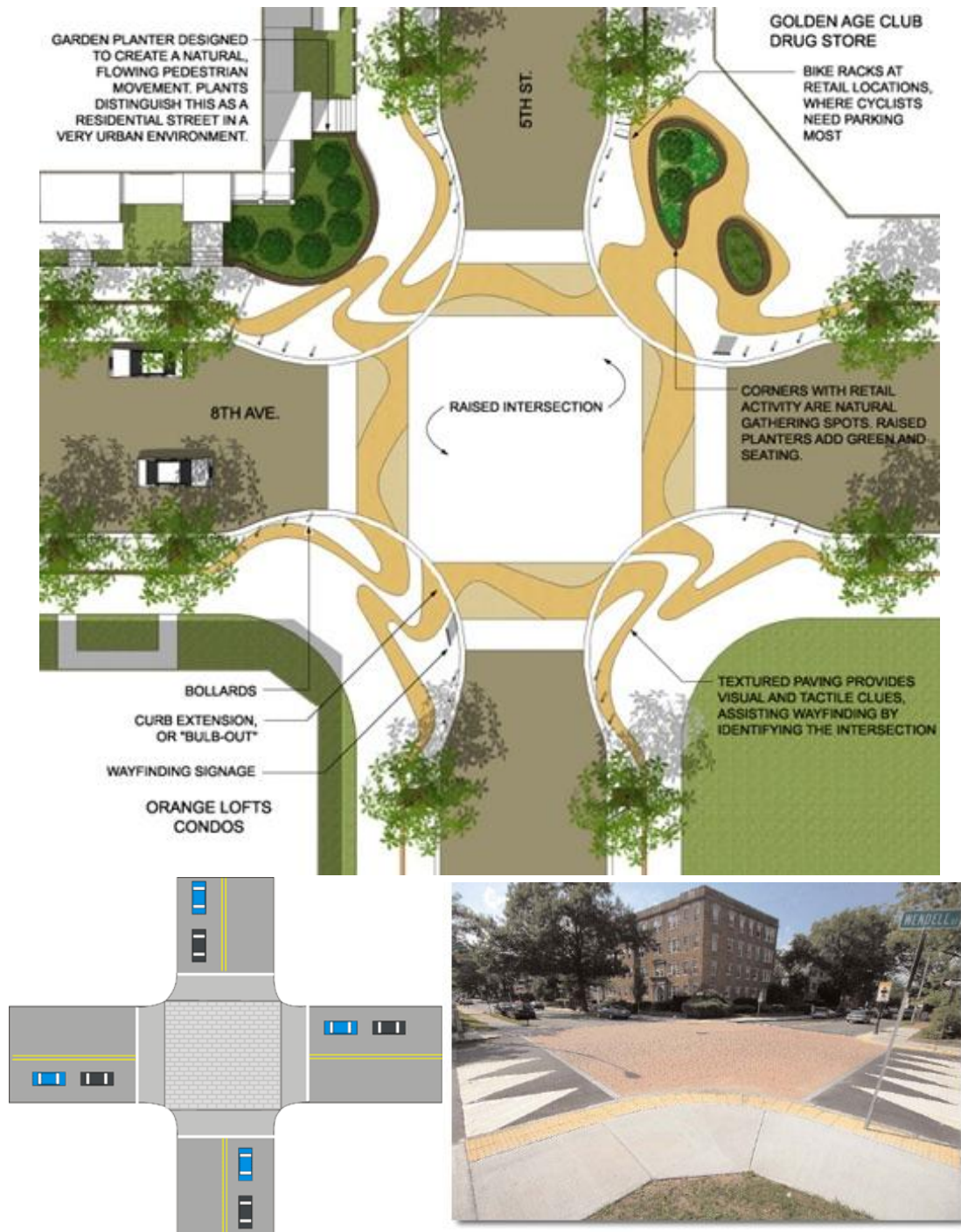
Figura 116 - Esempi di intersezioni rialzate (fonti: https://www.aiit.it/wp-content/uploads/2017/10/berloco_.pdf ; http://dpw.lacounty.gov/tnl/NTMP/Raised_Intersections.shtml ; http://apakatagemilang.blogspot.com/2014/ )
